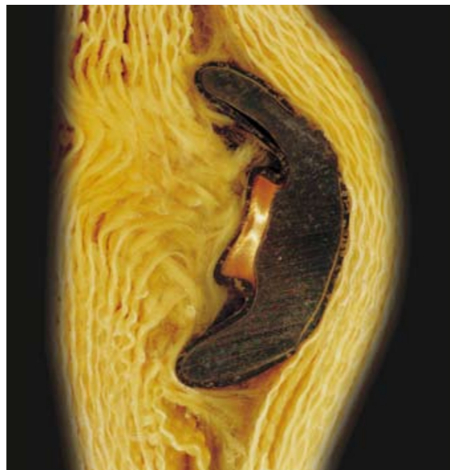
Cross-section of Twaron body armor showing trapped 9 mm bullet
