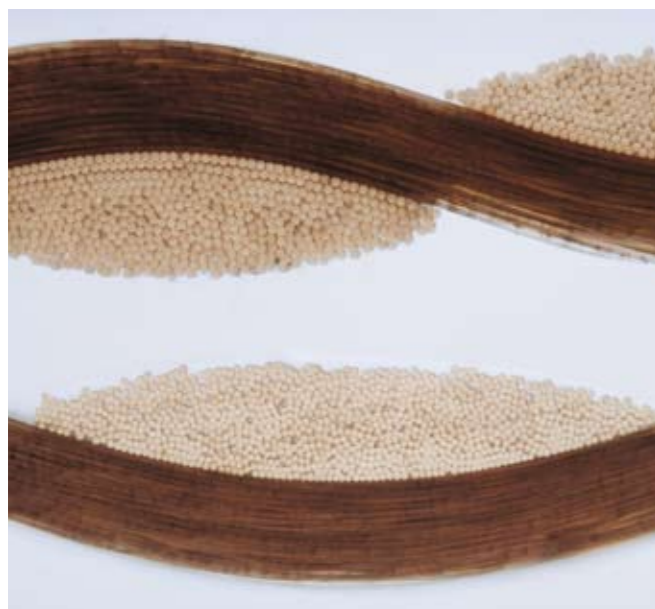
Cross-sections of standard yarn (above) and Microfilament (below)
